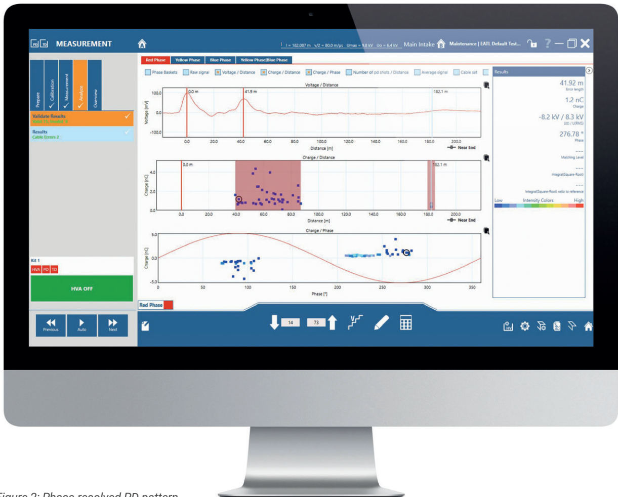
Figure 2: Phase-resolved PD pattern
