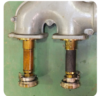
Intact and arced bushings
