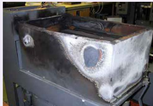
Explosion in 3.3kV circuit breaker.
