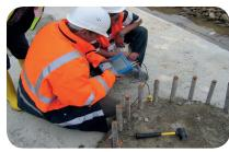
EA Technology offers a comprehensive range of on-site testing and analysis services utilising the measurement of Polarisation Resistance and Transient Dynamic Response (TDR) to assess the condition of tower foundations.
