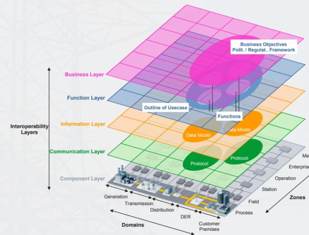
FIGURE 1. FIGURE TAKEN FROM "SMART GRID REFERENCE ARCHITECTURE," CEN-CENELEC-ETSI SMART GRID COORDINATION GROUP, NOV., 2012.\*
