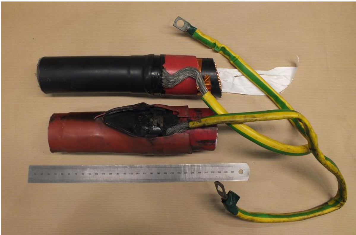
Figure 1. Samples supplied to EA Technology for examination. Non-failed termination is upper in the picture, failed termination is lower.
