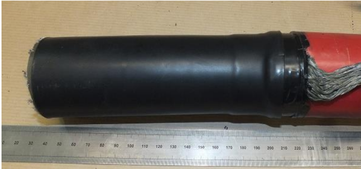
Figure 10. Non-failed sample, stress control tube in good condition
