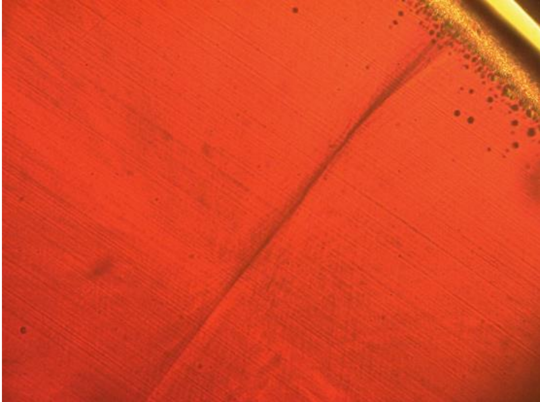
Figure 16. Non-failed sample: prominent extrusion seam in the XLPE
