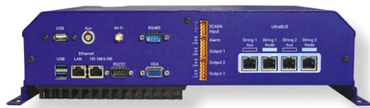
The Astute<sup>®</sup> HV Monitor is a fully integrated, modular system that collects data on the condition of HV assets through a cohort of specialised sensors. This scalable system consists of multiple multi-sensor nodes connected to a central processing hub for monitoring and alerts.
