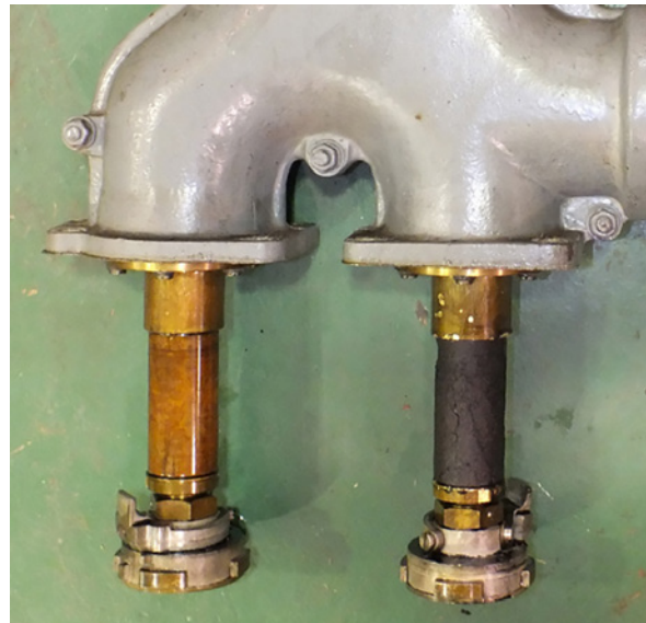
Intact and arced bushings
