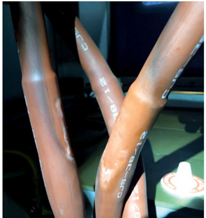
**Figure 1** Partial discharge caused by incorrect installation found on a cable termination using non-intrusive PD 'UltraTEV' instrument
