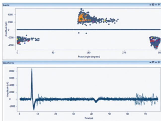
**Figure 5** On-line measurement of cable measuring partial discharge
