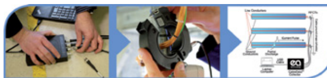
Figure 3 Equipment for 3-phase On-line measurement of cable PD
