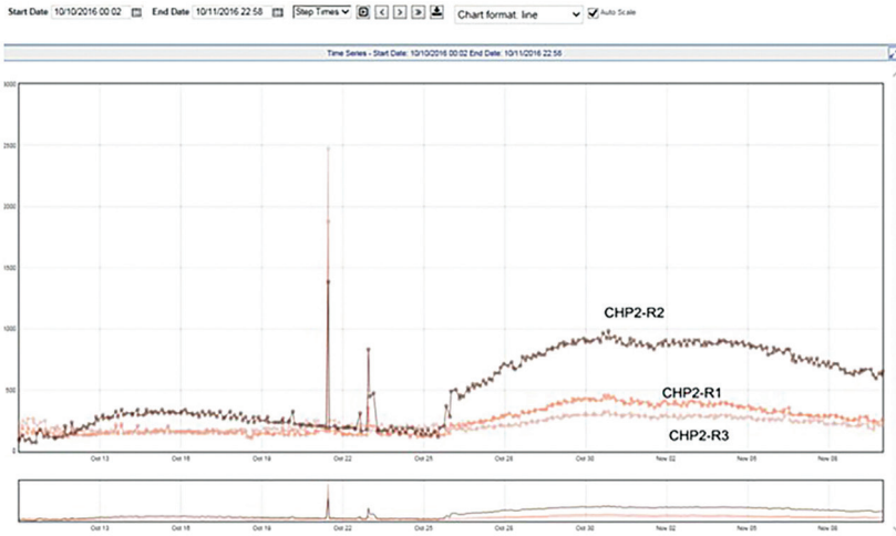
Figure 3: Rapid Increase in PD in CHP2-R2
