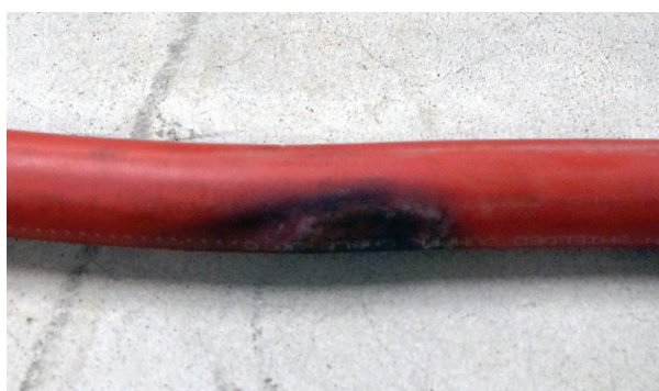
Figure 8: PD Damage to PT Cable
