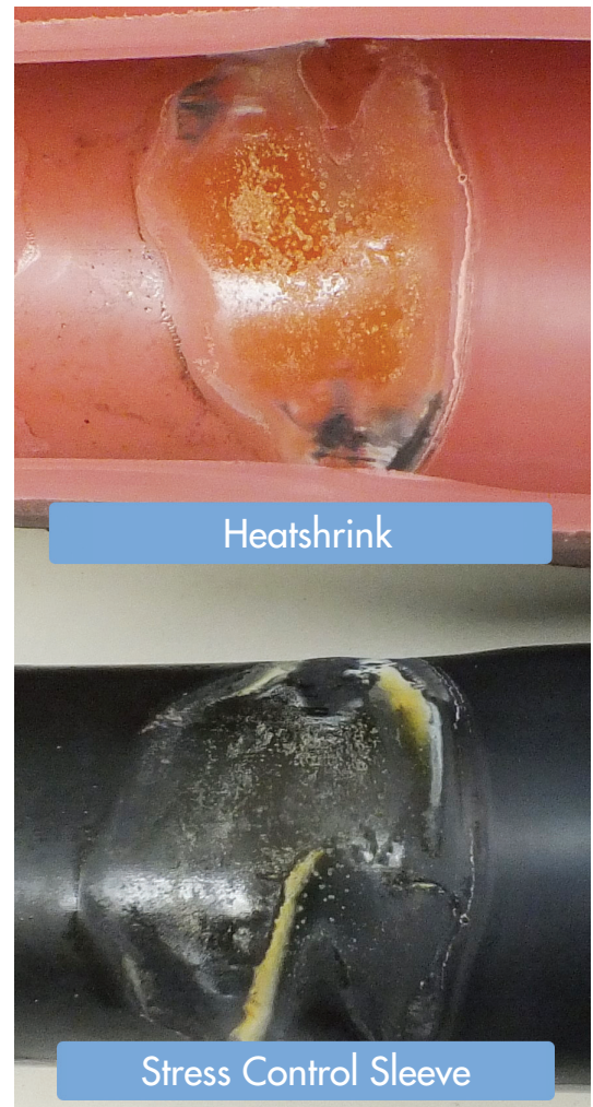
Figure 5: Partial Discharge Location
