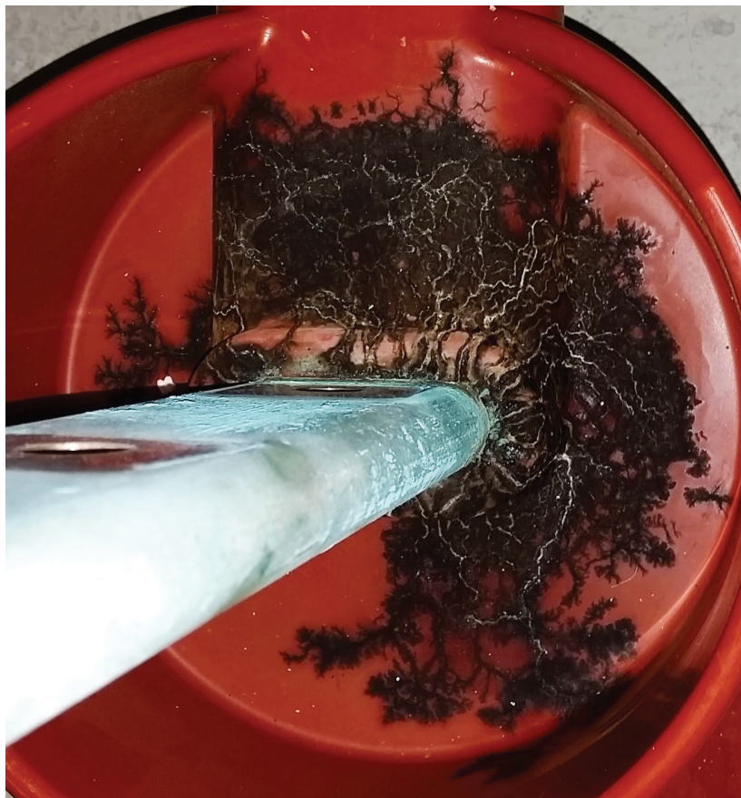
Figure 7: PD Caused by Excessive Saltwater Humidity
