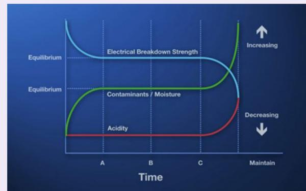
Schematic representation of oil condition parameters as a function of time (for oil filled switchgear).
