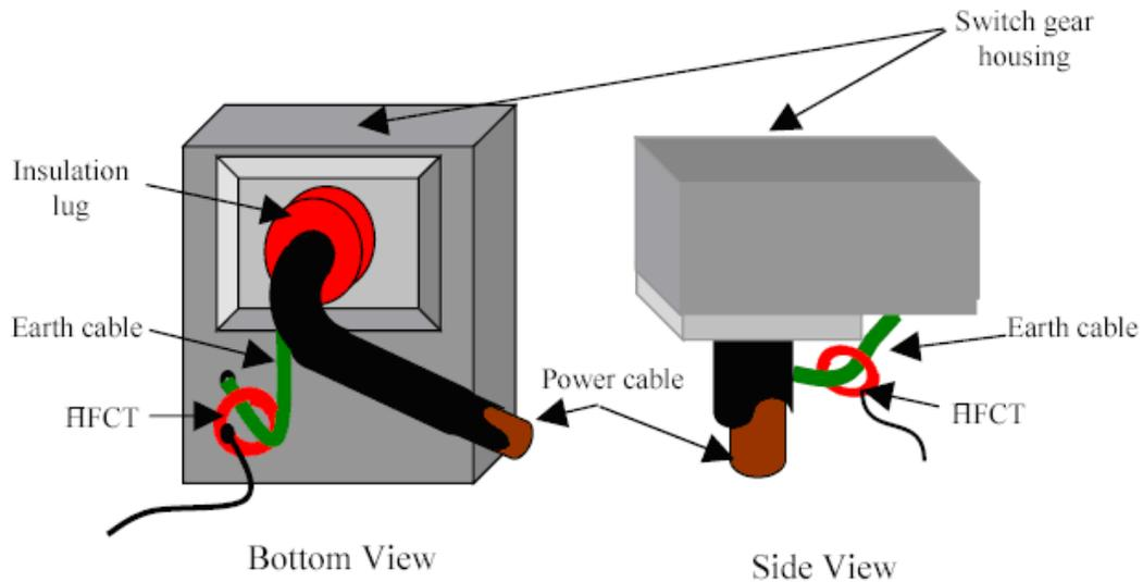
Figure 8. Connection point for RFCT on a 11KV Pad Mount Transformer
