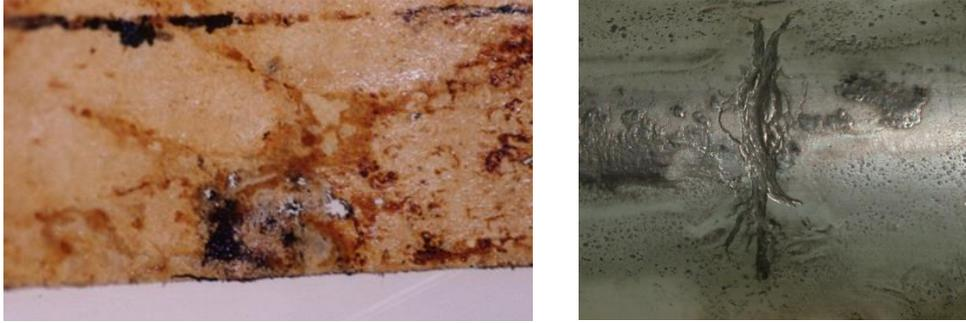
Figure 2. Degradation of cable insulation (left: paper, right: XLPE)
