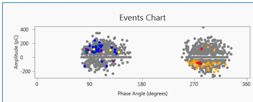
Figure 6. Phase-resolved plot showing true PD activity
