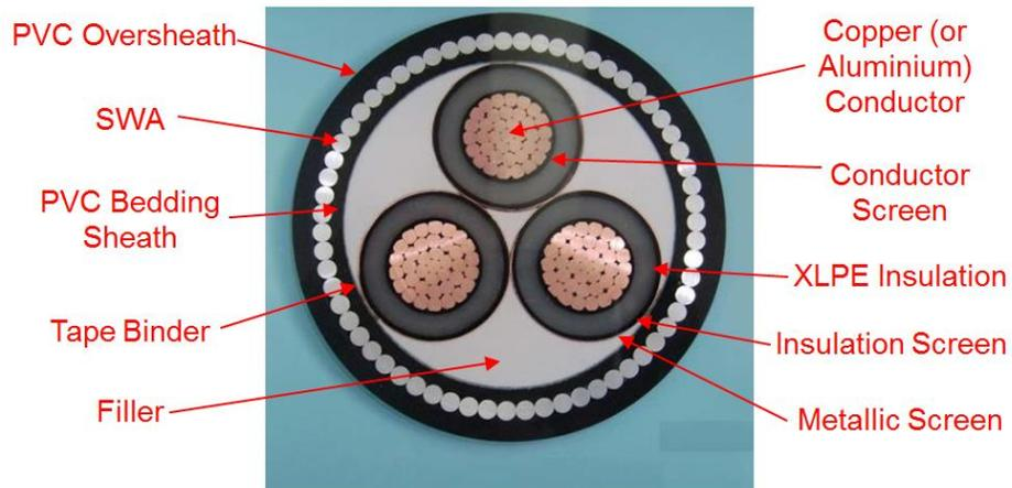
Figure 17. Typical cross section of 3-core XLPE cable
