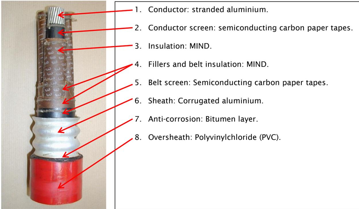
Essentially PICAS cable can be thought of as being functionally identical to PILCSWA, with the only physical difference being the lead and armour layers replaced with a corrugated aluminium layer. The same restrictions apply in that the phase on which any PD may be occurring cannot be differentiated.
