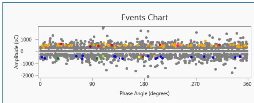
Figure 7. Phase-resolved plot showing background noise
