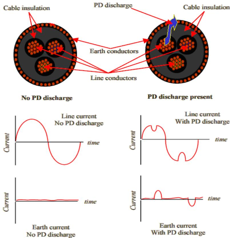
**Figure 3. Simplified representation of cable PD**
