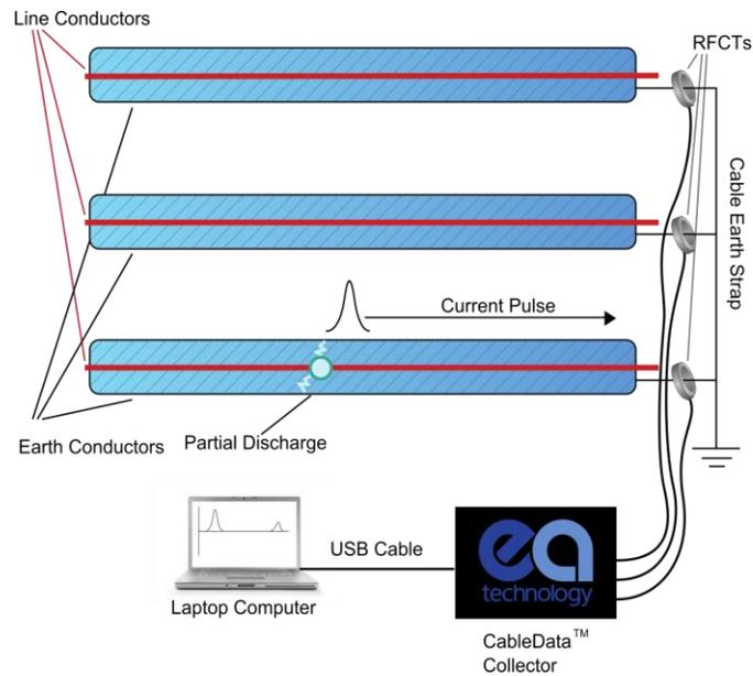
**Figure 4. Basic diagram of CDC operation**
