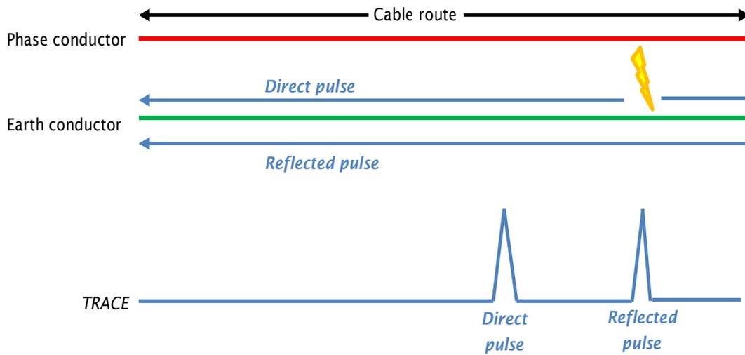
**Figure 5. Representation of time-of-flight principle for discharge location**
