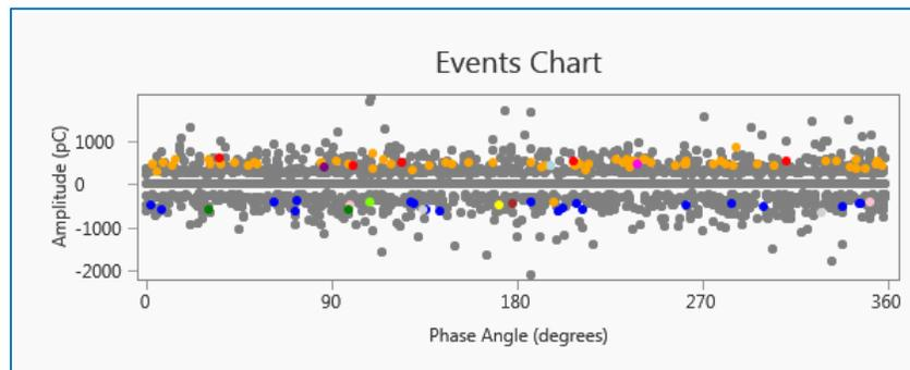
Figure 7. Phase-resolved plot showing background noise
