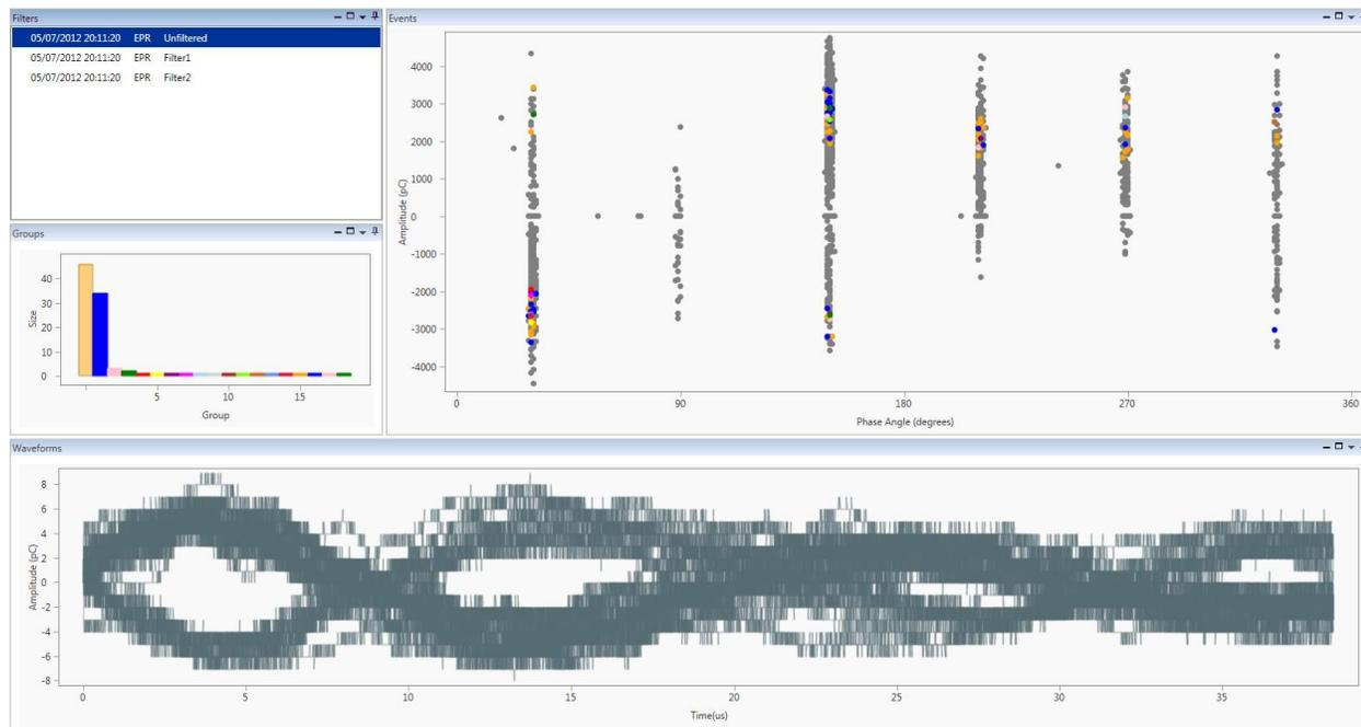
Figure 19. VSD/machine noise
