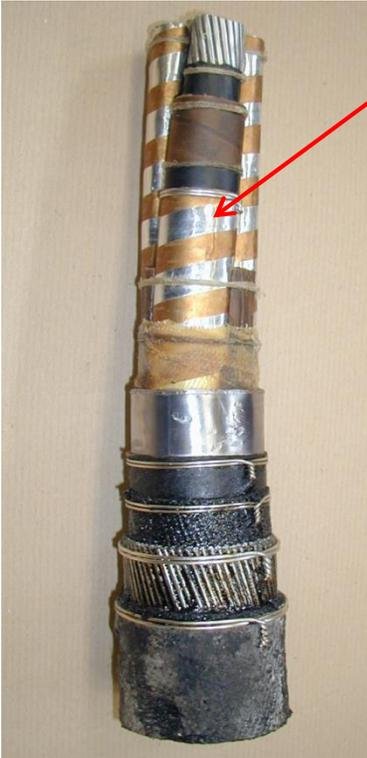
1. Note the only difference from normal PILCSWA is the presence of aluminium foil or copper tapes around each phase conductor's semiconducting layer.
