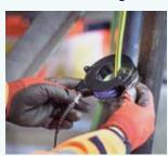
The CableData Monitor® allows us to continuously monitor and report to you on PD activity in live cable networks. This helps to reduce the need for disruptive maintenance shutdowns by highlighting high risk areas in ample time for repairs and
