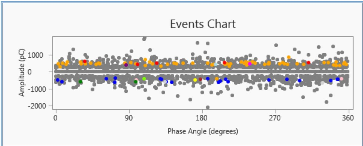
Following analysis of the events chart the waveforms associated with the coloured dots are analysed to determine if they are characteristic of partial discharge activity.
