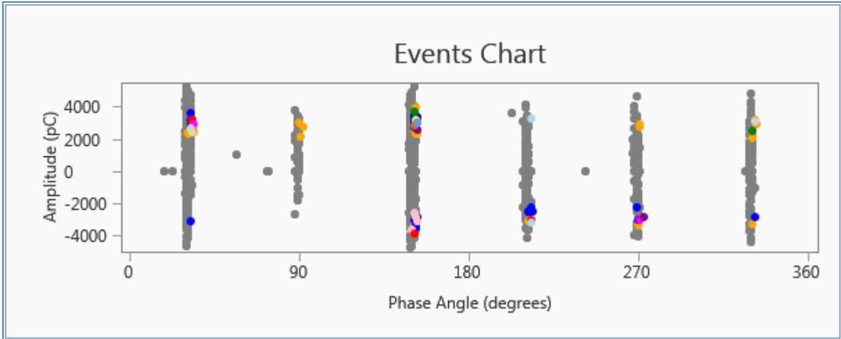
**Background interference:** - Easily identified as it occurs randomly on the phase event plot as it not referenced to the mains frequency. This may include activity from radio masts, DC light fittings etc...
