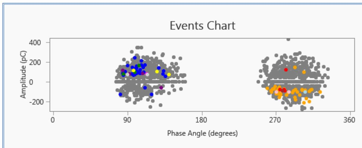
**Machine Noise:** - Generally caused by rotating machines characterised by tight linear stripes on the phase resolved plot.
