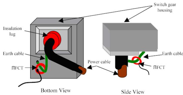
Figure 1: Cable CT Attached to Ground Strap
