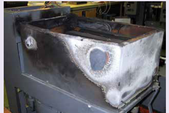
Explosion in 3.3kV circuit breaker.
