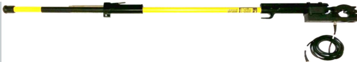
\* The RFCT Hot Stick is designed to keep the users hands and body away from accidental contact with dangerous voltages. Due to the RFCT cable, the hot stick does not isolate the CDC or laptop from HV. Once the RFCT is attached around a good ground connection, the cable should be at or near ground potential and therefore safe. For complete isolation please contact EA Technology LLC to learn about our fiber isolated Cable Data Collector.
