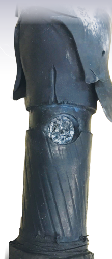
Figure 7: Failed EHV Termination
