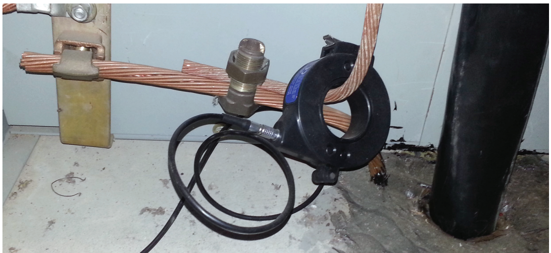
Figure 4: Properly Placed RFCT
