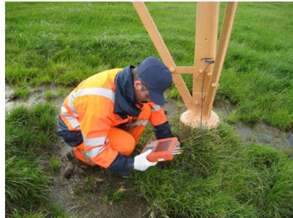
Figure 1: Polarisation resistance measurement
