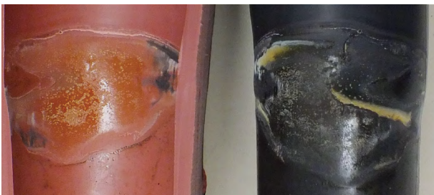
One of the three HV cables at the Grangemouth site where routine testing revealed critical PD activity.
