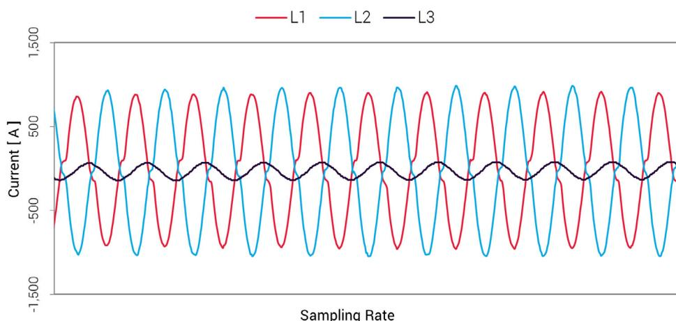
Figure 1: The current waveform of feeder 4 captured by VisNet<sup>®</sup>. The 'L' labels denote the feeder phase measured.
