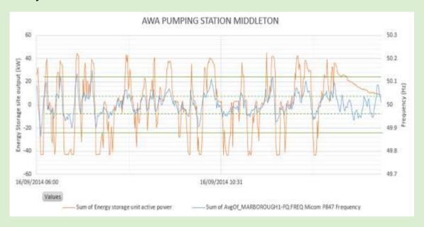
The chart above shows early operational experience of frequency regulation using the inverter and battery unit installed as part of FALCON, and frequency measured elsewhere on the network.
