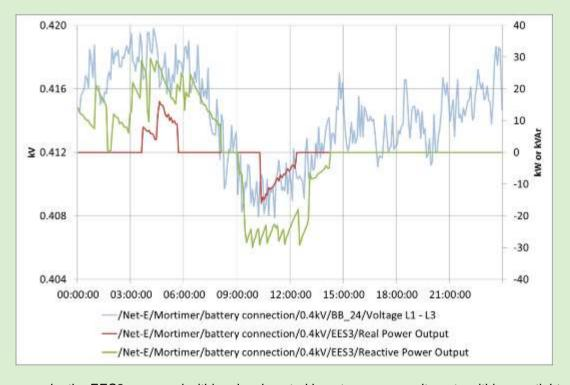
In this example, the EES3 was used within a local control loop to manage voltage to within very tight limits. The controller was set to use reactive power in the first instance to resolve voltage issues as this does not alter the SoC of the battery (i.e. leaving real power available to manage any thermal issues).
