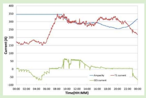
In this example, EES1 was used to ensure that the current supplied by the transformer did not exceed a maximum ampacity of 345A (1.5 times its static rating of 230A).
