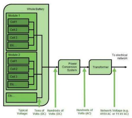
Figure 9.1: Block Diagram of EES with Approximate Voltages
