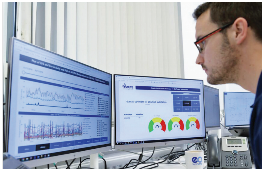
The system can monitor, record and analyse the condition of hundreds of assets simultaneously, including cables. Results are filtered to remove false alarms and clients are alerted of problems automatically.
