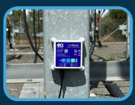
A phase lock is critical to understanding partial discharge in high voltage systems, enhancing data analysis and optimising decision making. The new wireless phase reference accessory guarantees an accurate phase lock in any environment.
