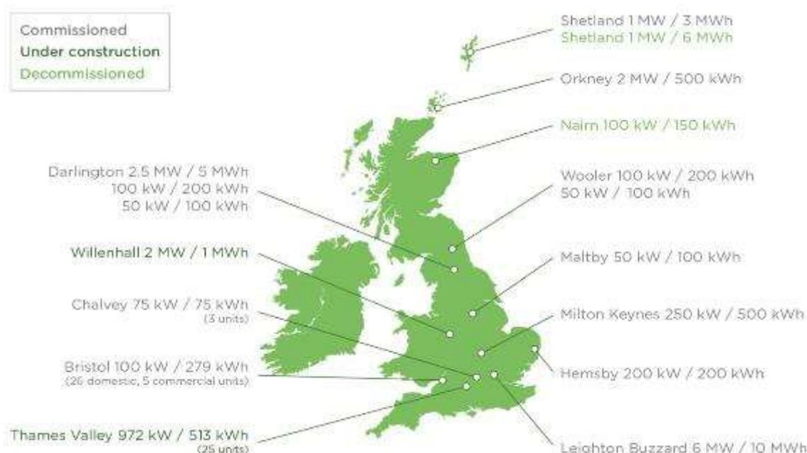
**Figure 2.4: GB DNO Deployment of Electrical Energy Storage (at 1<sup>st</sup> December 2014)**
