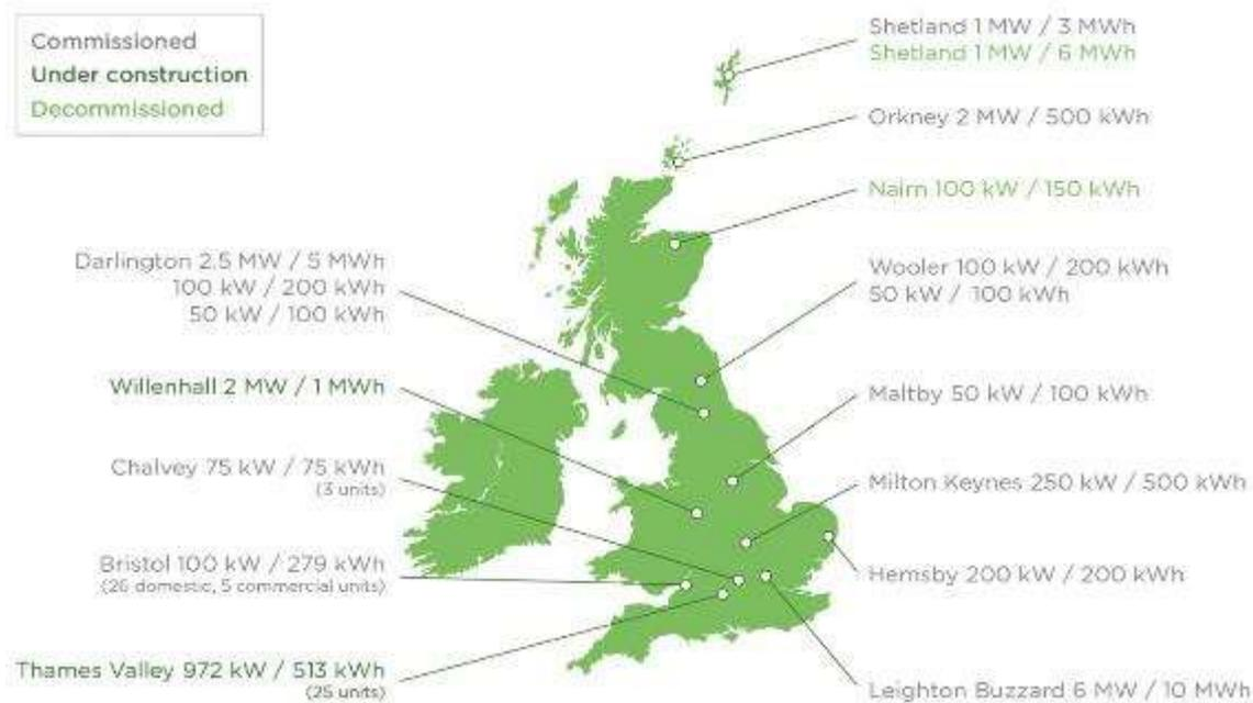
**Figure 5.1: Deployment of Storage in the UK (at 1<sup>st</sup> December 2014)**
