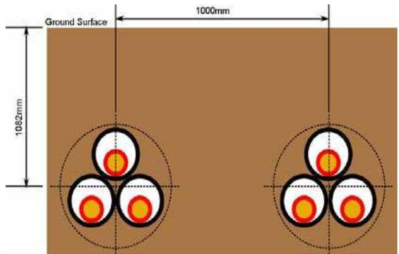
Figure 1: Duct Laying Centres: Trench Profile
