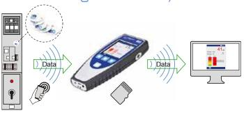
The UltraTEV Plus² has Near Field Communication (NFC) capability to store Asset data on programmable tags. It also has the ability to transfer the results directly on to your PC or business network, via Wifi or USB/SD Card. The new survey functionality allows details of substations and assets to be entered on the screen and guides users through the simple survey process. Screen shots can also be captured and saved.
