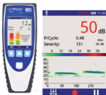
TEV interpretation screens include Phase Resolved view to discriminate between PD and noise.
