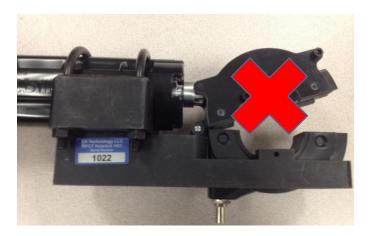
Never allow hinged portion of the hotstick to take a load on the cable ground.
