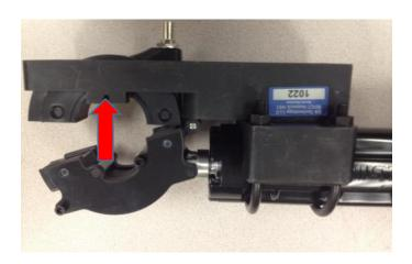
Correct positon for load from a ground wire.
